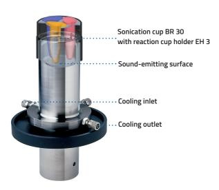
It functions like a "mini high-performance ultrasonic bath". The sample material is enclosed in a sealed vessel and is sonicated from outside via a transfer medium (e.g., iced water). The transmitted power density [W/I] is approximately 150 times higher than in a "normal" ultrasonic bath, but lower than with direct sonication with a probe.
