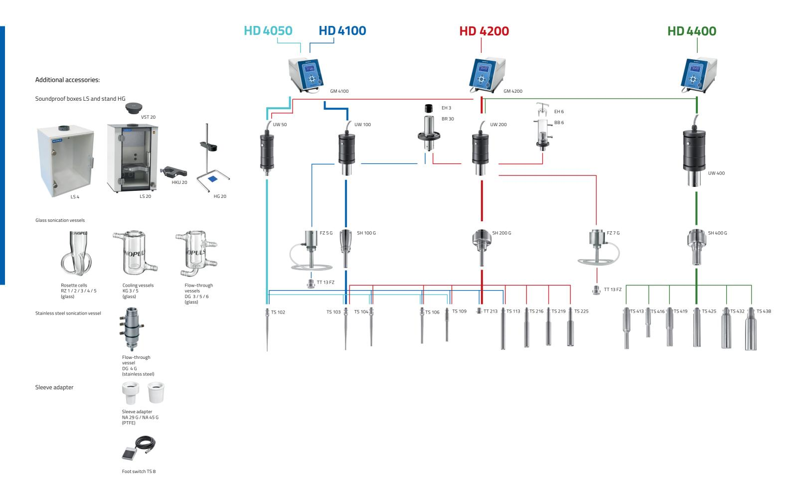
Stainless steel or glass sonication vessels and sleeve adapters depend on the ultrasonic homogeniser used and the probe.
