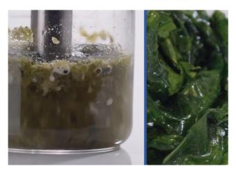
In the case of plant cells, up to 15 min are needed since the cells possess one additional shaping membrane. Thermal damage to the cell contents can be prevented by employing pulsation, i.e., periodic interruption of the power supply. In addition, respectively suitable time intervals can be set on the device. Cooling down is possible during the pulse pause.
