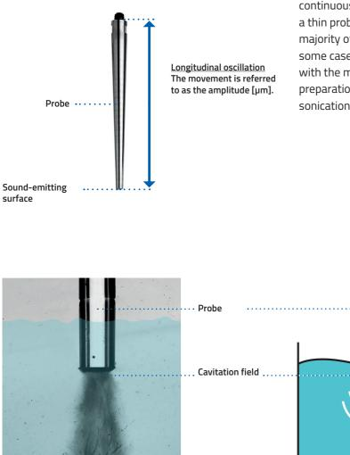
The smaller the diameter of the probe tip, the higher the power density and cavitation power for the same electrical power consumption! The sonic distribution conforms to a row of "hemispherical shells" increasing in radius the further they are from the sound-emitting surface (see diagram below). The power density decreases at the same time.
