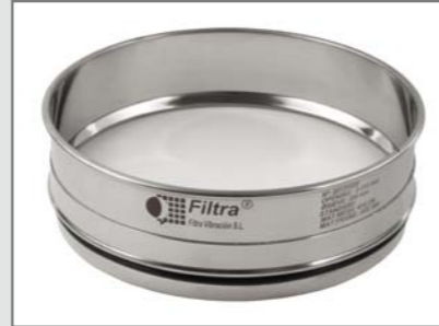
Stainless steel framed sieve with nylon mesh.
