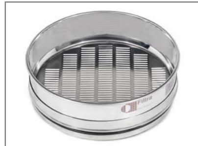
Stainless steel sieve with oval-holed perforated plate (for cereals, ISO 5223).
